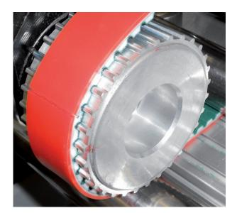
When general conveying and precision product placement are in demand, timing belts take on the same challenges as conventional flat belts. One challenge has always been to develop a process for changing belts quickly. Normally, to replace an endless timing belt one would need to tear down the conveyor system and outboard components or joint the belt endless on the system. Both take time and lead to costly lost production.
